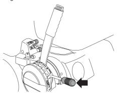
It is important that the air pressure in both front wheels is equal, 60 kPa / 0.6 bar / 8.5 PSI, to produce an even cutting height.
